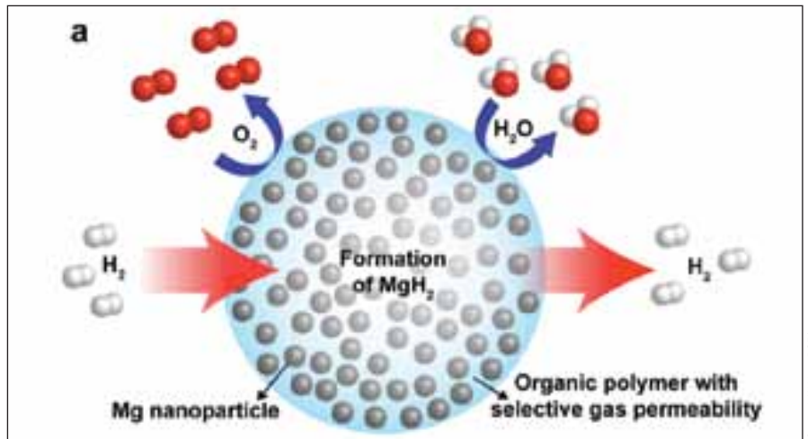
Berkeley lab's schematic of how high-capacity magnesium nanocrystals encapsulated in a gas-barrier polymer matrix provide a new and revolutionary hydrogen storage composite material.
