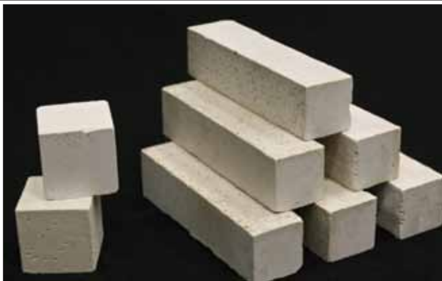
Blocks made with Novacem cement.
