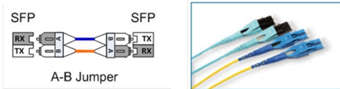
Figure 1: Duplex Fiber Optic Transmission
